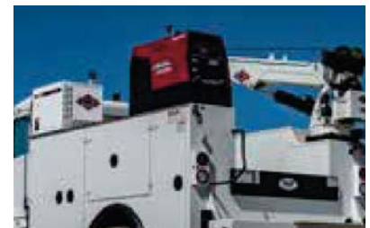
IMT CAS45 COMPRESSOR AND IMT 10000 CRANE
