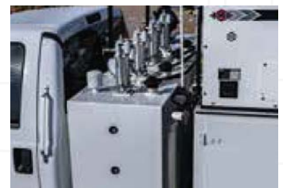
LUBE DECK - LUBE, OIL AND RECOVERY SYSTEM
