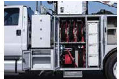
LUBE, OIL AND RECOVERY SYSTEM WITH REELS
