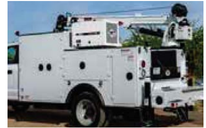
IMT 7500 CRANE AND CAS40 COMPRESSOR
