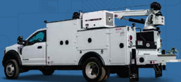
Service Truck with Weld Deck and Crane
