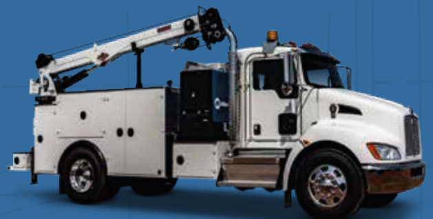
Service Truck with Weld Deck and Crane
